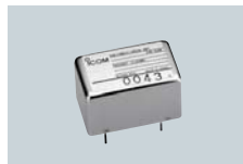
CR-338 HIGH STABILITY CRYSTAL UNIT Contains a temp. compensating heater for improved frequency stability. Frequency stability: \pm 0.5 ppm
